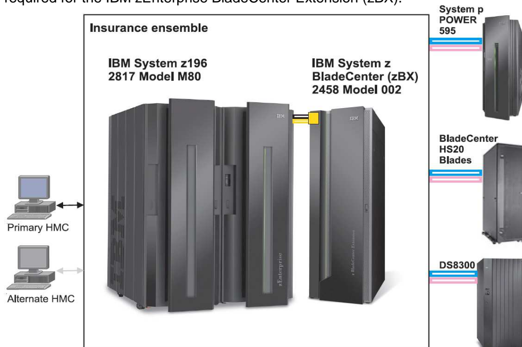
Figure 2 The Insurance Company hardware configuration with zEnterprise components
