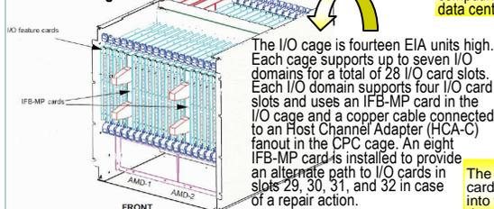
The I/O cage is fourteen EIA units high. Each cage supports up to seven I/O domains for a total of 28 I/O card slots. Each I/O domain supports four I/O card slots and uses an IFB-MP card in the I/O cage and a copper cable connected to a Host Channel Adapter (HCA-C) fanout in the CPC cage. An eight IFB-MP card is installed to provide an alternate path to I/O cards in slots 29, 30, 31, and 32 in case of a repair action.
