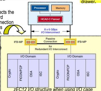
zEC12 I/O structure when using I/O cage
