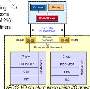
zEC12 I/O structure when using I/O drawer
