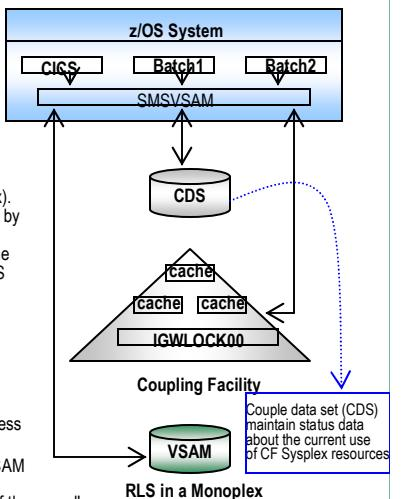
VSAM internally performs cross-address space accesses and linkages between requestor address spaces and the SMSVSAM server address space. The SMSVSAM server owns two data spaces. One data space is called the SMSVSAM data space. It contains some VSAM RLS control blocks and a system-wide buffer pool. The other data space is used by VSAM RLS to collect activity monitoring information used to produce SMF records.
