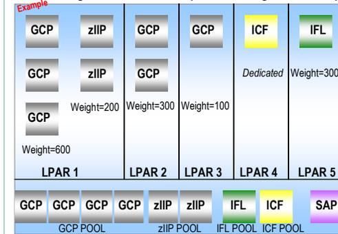
Typically in most cases PR/SM will manage the processing weights to within 1% of the LPAR's physical per CP share.
